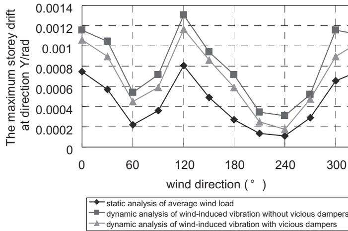
Figure 9. Comparison of maximum storey drifts under different wind directions
