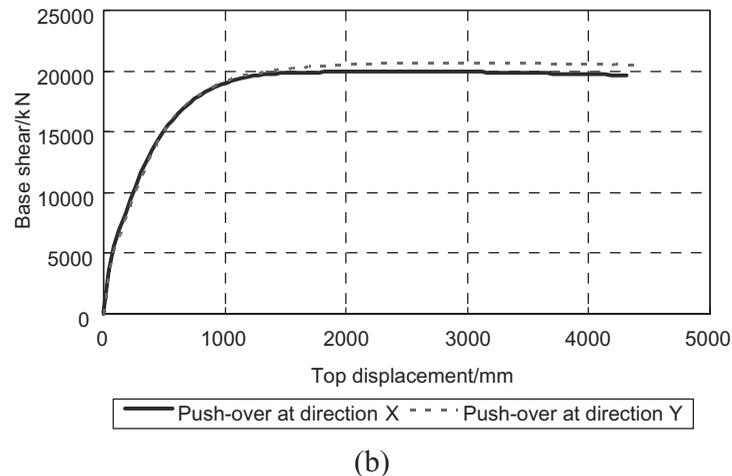
Figure 8. Top displacement–base shear curve: (a) the left tower and (b) the right tower
