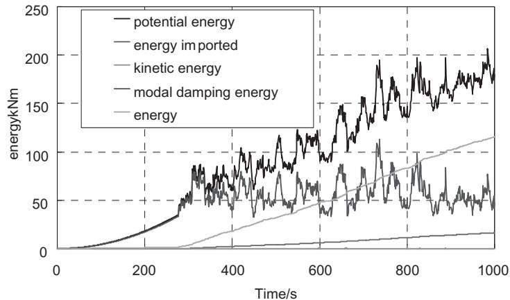
Figure 11. Structural energy dissipation curve of dynamic wind load under direction  $0^\circ$
