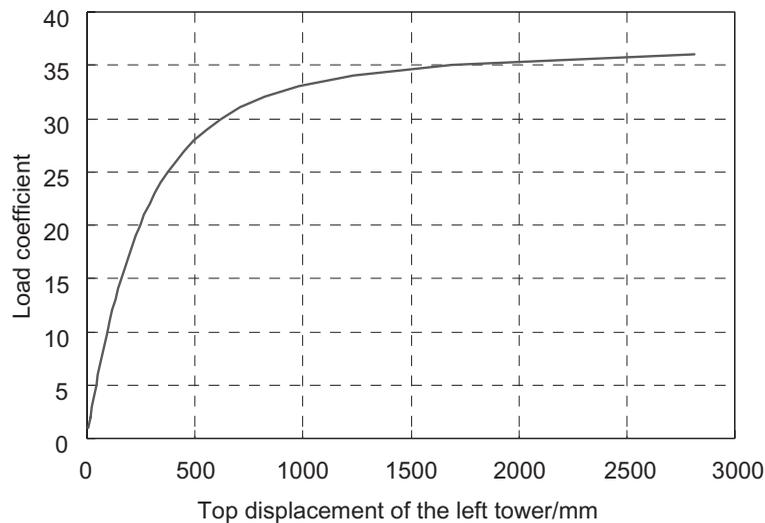
Figure 7. Load coefficient–top displacement curve of the left tower
