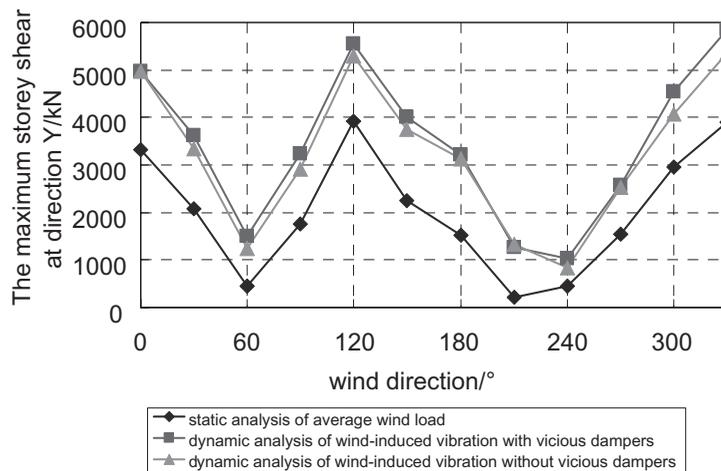
Figure 10. Comparison of maximum storey shears under different wind directions
