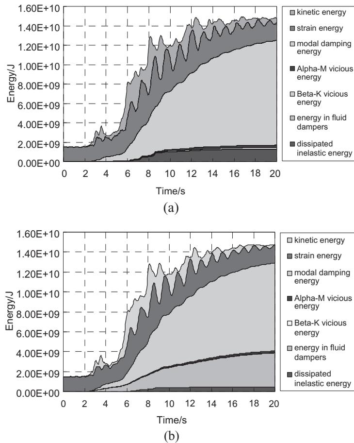
Figure 14. Energy dissipation: (a) take no consideration of dampers, and (b) take consideration of dampers
