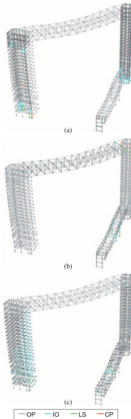
Figure 13. Performance of elements under condition GM3Y: (a) shear walls, (b) frame columns and steel brace and (c) frame beams and steel beams
