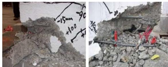
Fig.16 Local collapse of specimen 1
