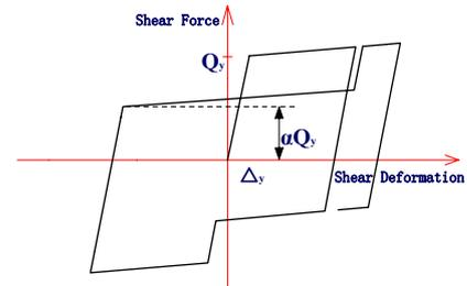
Fig.4 Restoring force model of horizontal shear
