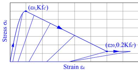
Fig.9 Kent Park modified concrete model(1982)
