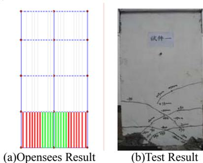
Fig.15 Comparison of collapse status of specimen 1 between FEA and experiment
