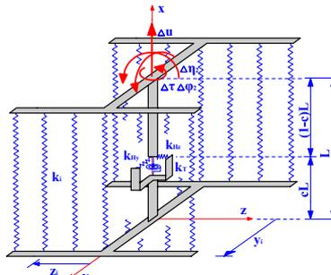
Fig.3 Sketch of MVLEM3D element
