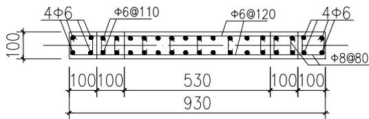
Fig.5 Dimension and details of Spec.1 and Spec.2
