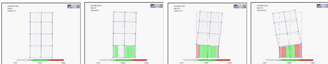
Fig.14 Collapse process of shear-wall elements shown in SWNA
