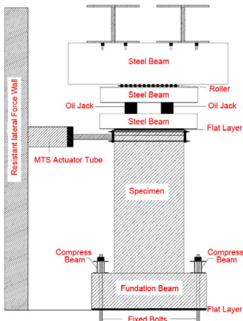
Fig.7 Figure of experiment device
