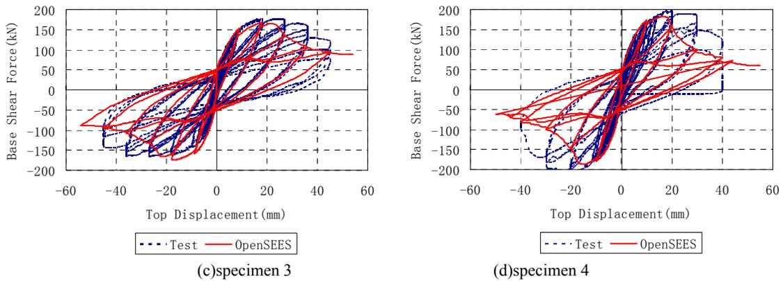
Fig.12 Comparison of force-deformation curve between experiment results and OpenSEES
