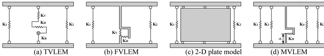
Fig.1 Macro model of shear wall
