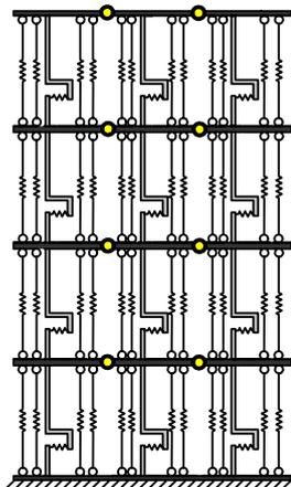
Fig.10 Finite element model of specimen
