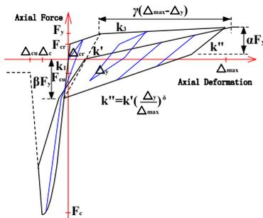
Fig.2 Restoring force model of vertical spring
