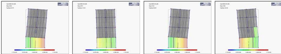
Fig.13 Deformation of vertical springs of shear-wall elements
