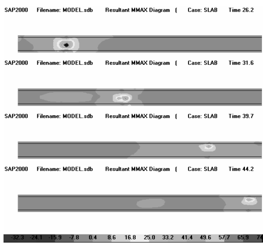
Fig.7 Moment response of floor system (N=1)
