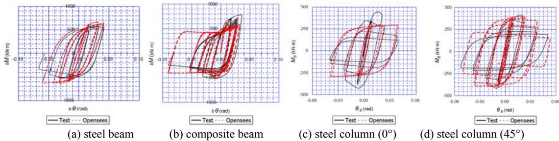
Figure.8 comparison of M- $\theta$  curve
