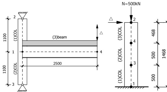
Figure.7 Simulation of the Steel Beam and Composite Beam under Cycle Loading
