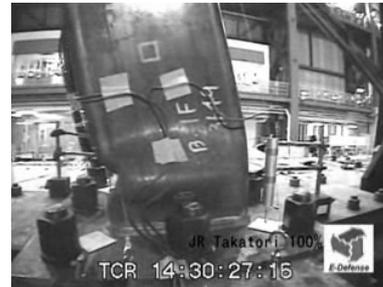
Fig.12 Photo Shot of Collapse      Fig.13 Local Buckling of Column End
