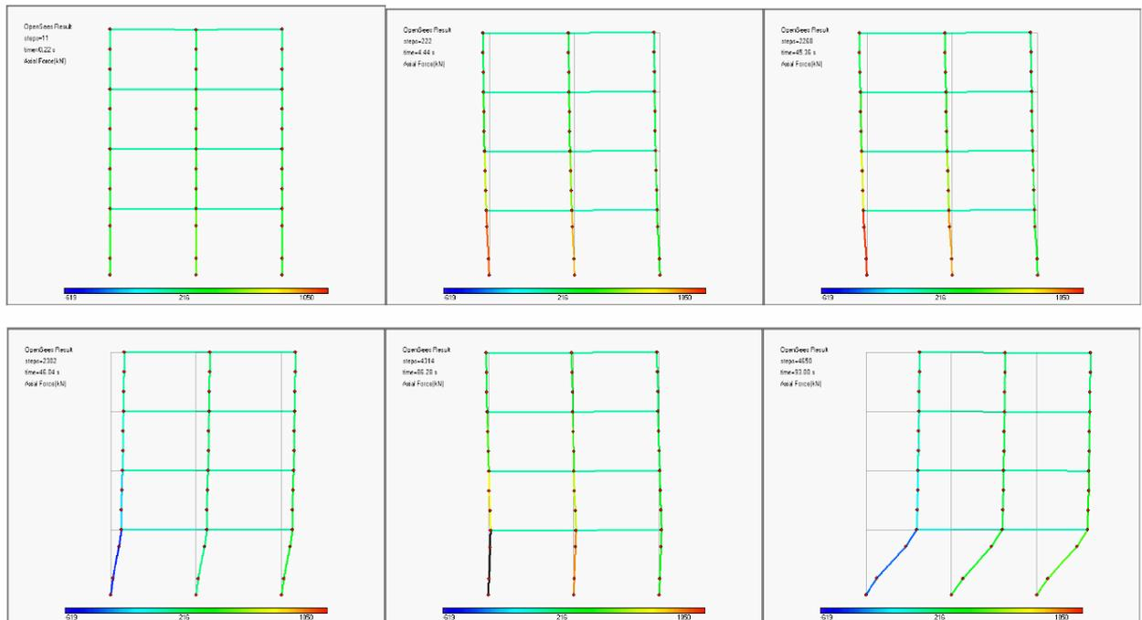
Fig.14 Deformation of Collapse in OpenSees
