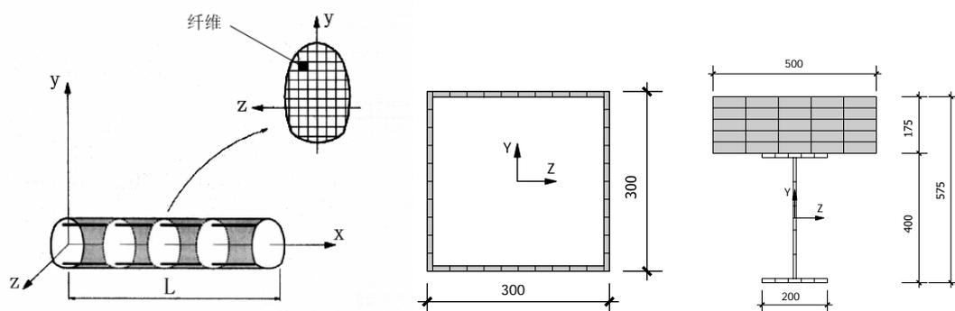
Figure.4 fiber element in local coordinates Figure.5 Fiber Section of Column Figure.6 Fiber Section of Composite Beam
