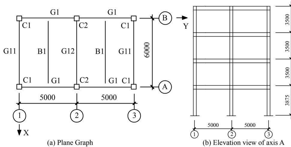
Figure.1 Framing Plan and Elevation of the Specimen
